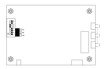
Strapping/DIP switch setting for DCF-radio (2 –wire) computer board
