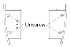
Remove the front and mount the back plate on the wall, using 4 screws suitable for the wall. We recommend Ø4mm and 30mm long screws.
