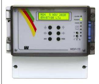
The WDP-AMP is an electronic quartz Impulse Amplifier for operating and control of analogue and digital Slave Clocks.
