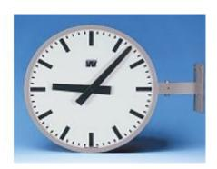
Westerstrand analogue clocks type **TIME CODE** are operated and controlled by serial time code (containing information about year, month, day, hour and minute) from Westerstrand Master Clock with time code output. This type of Master Clock provides, in combination with the time code, also 24VDC supply to the analogue clocks.
